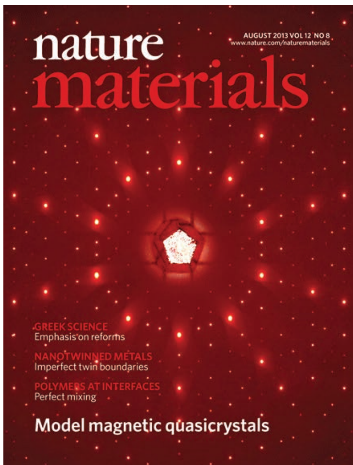
The cover of Nature Materials showing a high-energy x-ray diffraction pattern from a single grain of icosahedral rare-earth-cadmium quasicrystal, taken with x-ray beam from the APS superconducting undulator at beamline 6-ID-D.
