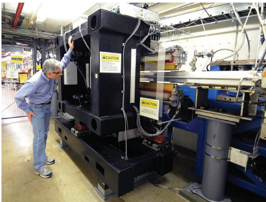
Kevin D'Amico, DCS Project Manager, with the newly installed prototype revolver undulator at Sector 35 in the APS storage ring.
