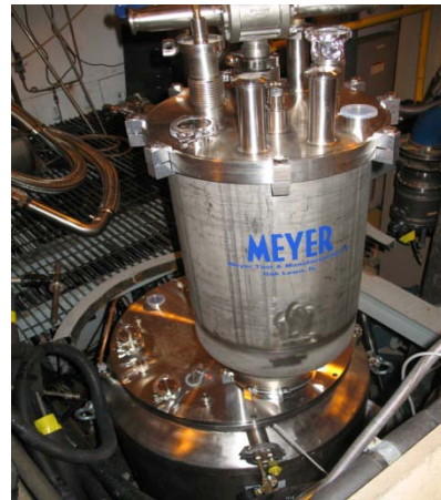
Cave platform showing 24" dewar with feedbox (left) and cryoplant connection box (lower right)
