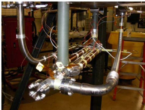
Three-channel test assembly installation.
