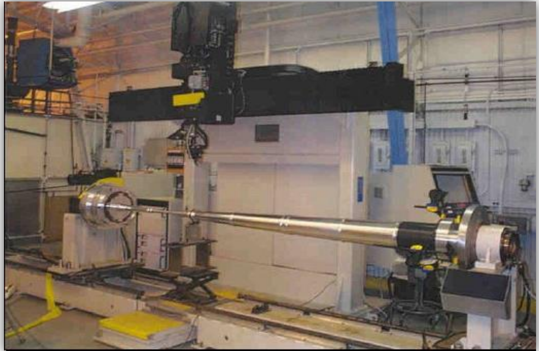
Fermi Numi Horn fabricated at Argonne using innovative welding methods to assemble and straighten the Numi Horn for Fermi lab Neutrino Experiment
