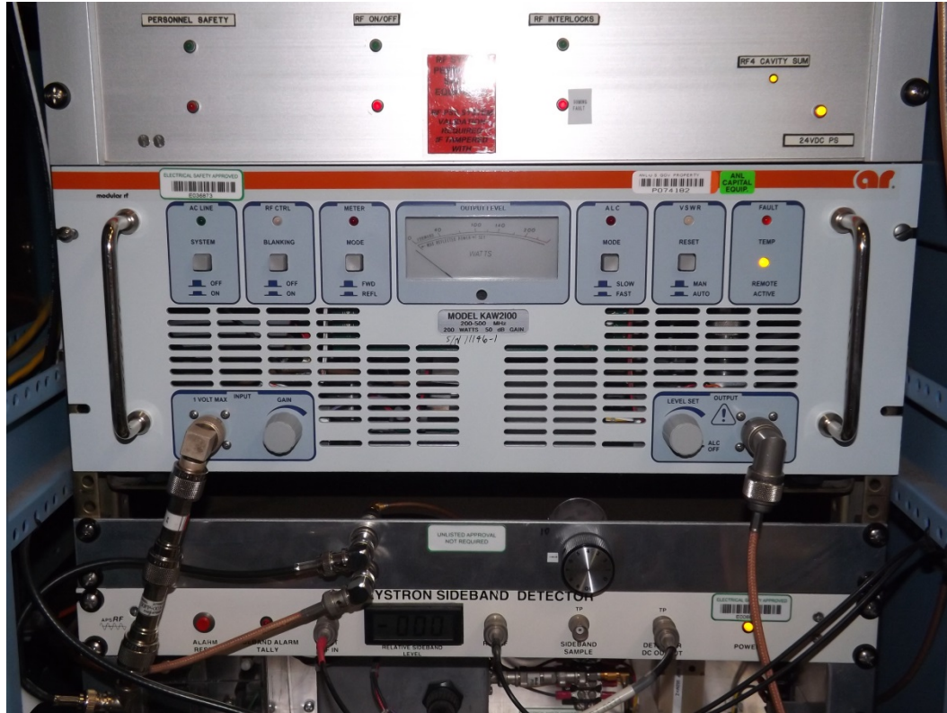
NEW KLYSTRON DRIVER AMPLIFIERS TO REPLACE OBSOLETE ORIGINAL UNITS
