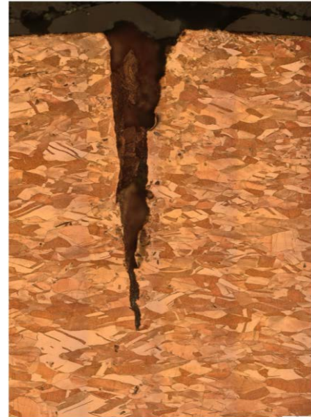
Metallurgical section of laser 100 μm drilled hole in copper
