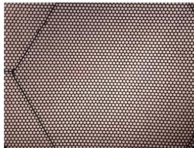
20 \mu m pore borosilicate MCA with 65% open area
