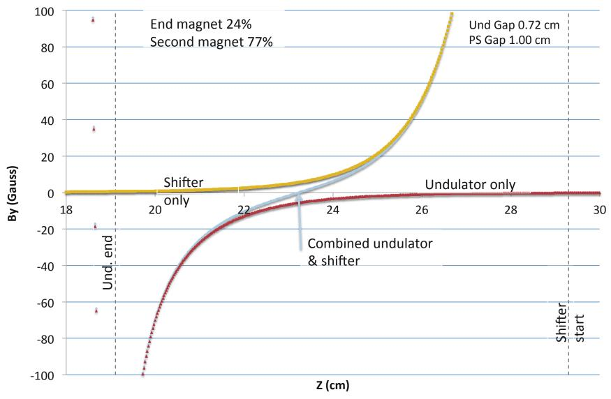
At 23.2 cm, the magnitudes of the shifter field and of the undulator field cross at 5.6 G. That's 4.12 cm from the undulator and 6.08 cm from the shifter.
