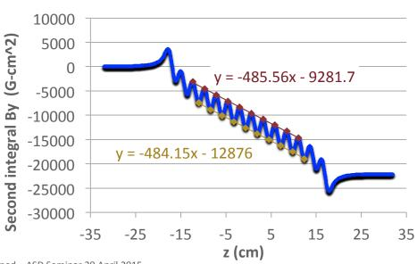
Magnetic design calculations for an undulator end, a phase shifter, and both combined. ASD Seminar 29 April 2015
