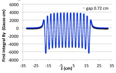
The 1<sup>st</sup> integral (angular kick) is zero after the undulator – by symmetry due to the even # of poles. Calc gives -8.5 G-cm (with attention paid to maintaining symmetry in the model). LCLS reqt: ±40 G-cm. APS goal:<50 G-cm
