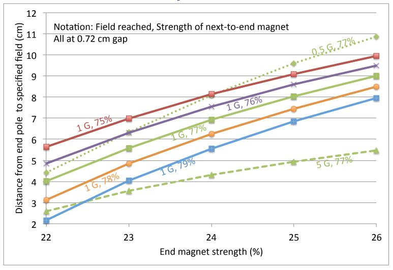
Field extends farther for stronger end magnet, and for weaker next-to-end magnet.
