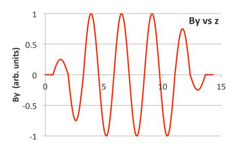
Now both the trajectory angle and the trajectory oscillate about zero, the trajectory is parallel to the undulator axis, and there is no offset.
