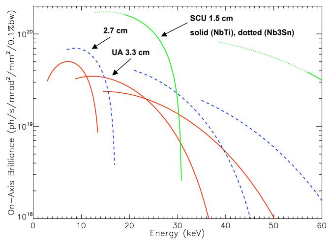
Superconducting undulators (SCUs) operate at a pole gap of 8 mm. The assumed magnetic fields on axis are 0.8 T for NbTi and 1.2 T for Nb<sub>3</sub>Sn (all lengths 2.4 m).
