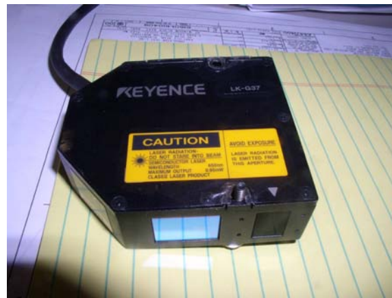
Keyence Proximity Sensor, 50 nm resolution
