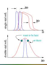
Monochromator Stabilizer Feedback loop to maintain constant detuning or beam position
