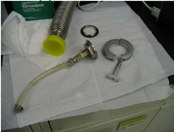
Figure 1: Special adapter for the Mar165 vacuum port. It is basically a vacuum hose attached to standard vacuum equipment.
