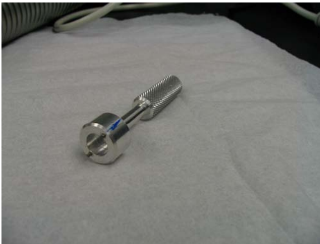
Figure 2: Vacuum valve key. This comes with the Mar165 toolkit. It is used to open the VAC VALVE on the mar165.
