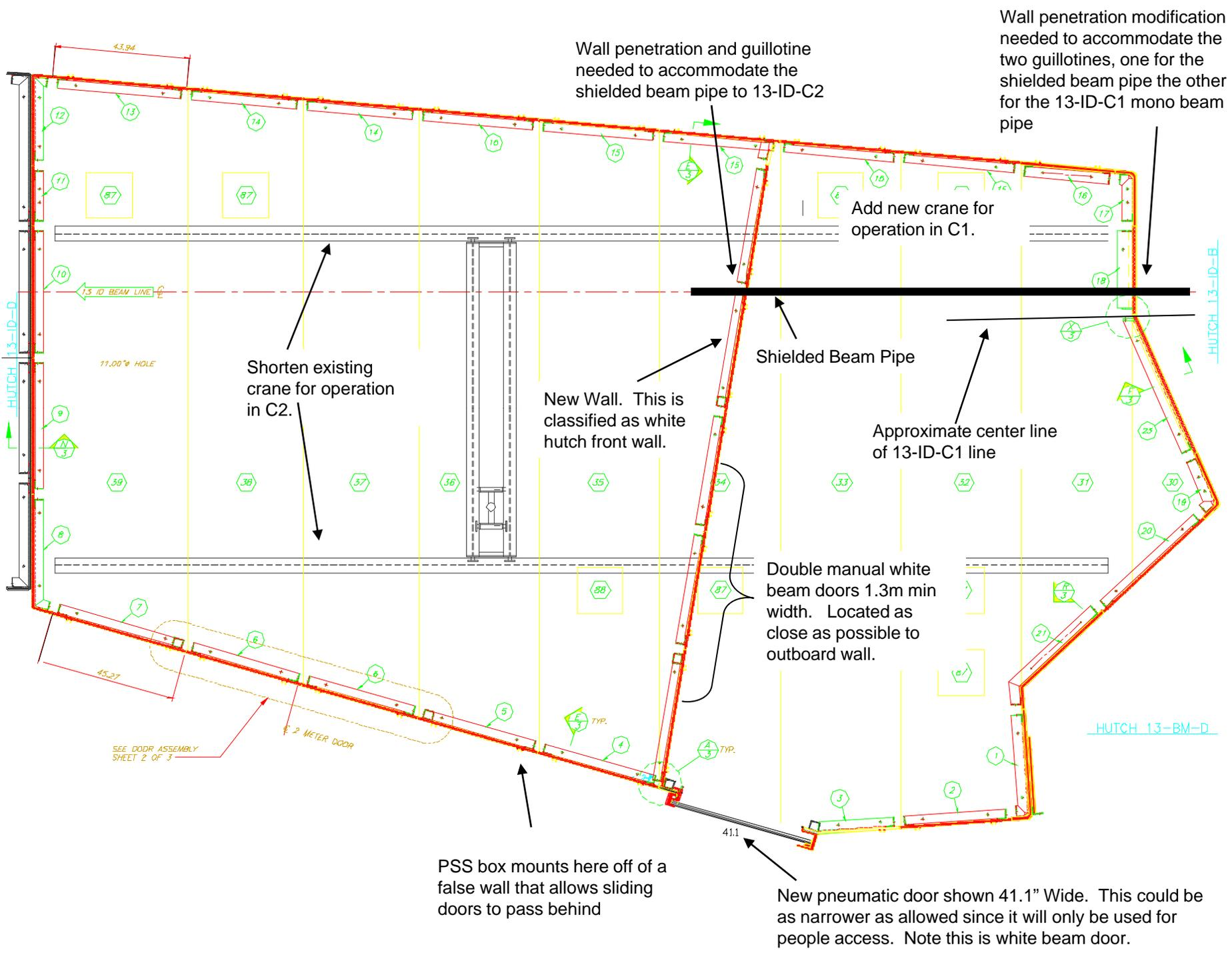
Wall penetration and guillotine needed to accommodate the shielded beam pipe to 13-ID-C2
