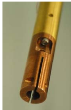
A custom-made Hall probe holder attached to a cold finger
