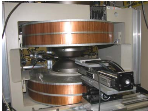
Electromagnet with a set of NMR probes
