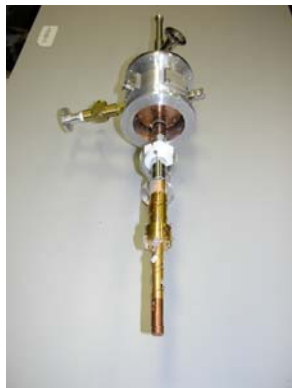
Janis cryostat with vacuum jacket removed
