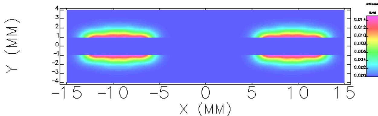
XRF Power by CU Flux through 0.1x0.1 mm<sup>2</sup> Pinhole
