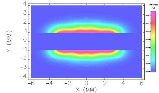
ID XRF Power by Flux through 0.1x0.1 mm<sup>2</sup> Pinhole
