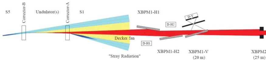
Figure 1: Top view of the undulator and XBPM showing the main design idea of GRID-XBPM and XBPM2.
