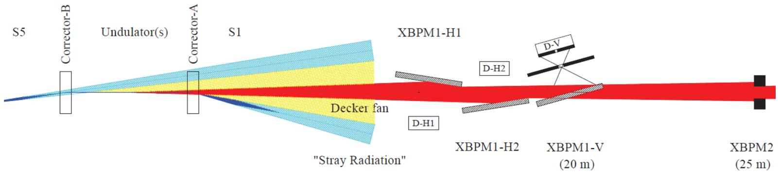
Figure 1: Top view of the undulator and X-ray beamline showing the main design idea of GRID-XBPM and XBPM2.
