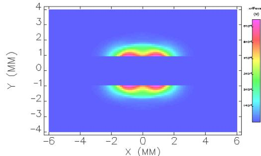
ID XRF Power by Flux through 0.1x0.1 mm<sup>2</sup> Pinhole
