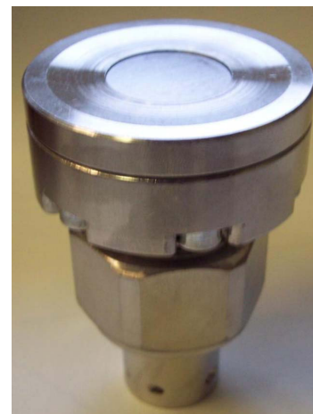
Electrochemical cell for Operando XRD and Mössbauer studies developed by Leriche et al. ( J. Electrochem. Soc. Vol. 157 (2010))
