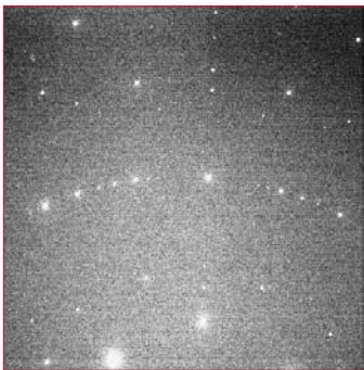
Figure 5. A microLaue image from a strain-free, thin-Si sample. The CCD-to-sample distance is 45 mm. The point-spread function is approximately 1.5 pixels FWHM. Image collected by Wenjun Liu (ORNL) on beamline 34-ID-E.
