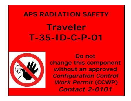
This is an example of a pre-installation tag for a device that designates where it will ultimately installed ((35-ID-c).
