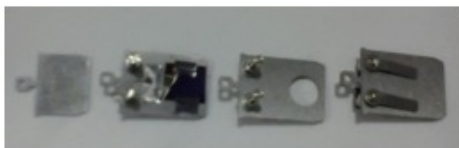
Available Omicron style sample holders, from left to right: Standard; Integrated thermocouple; Integrated thermocouple with hole; Biasing across surface or from surface to ground. All are made from molybdenum.
