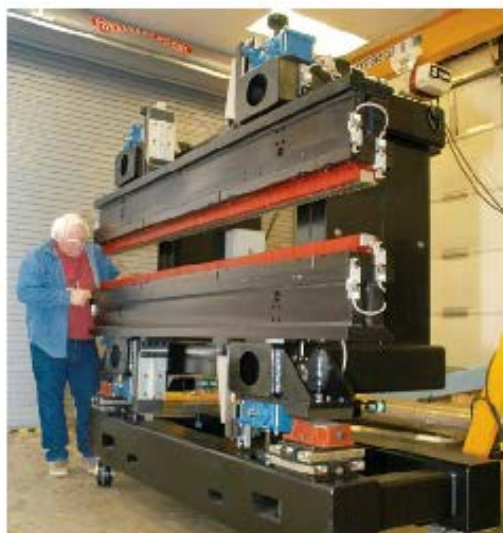
Planar Undulator Most installed IDs will be of this type.
