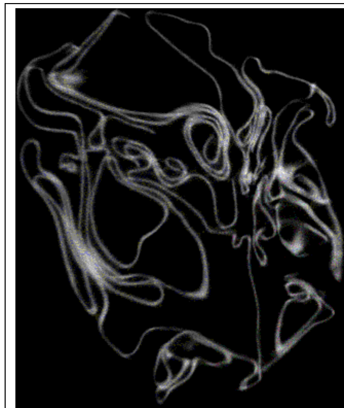
Figure 1: An XMT slice of a crumpled membrane.
