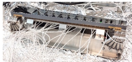
Fig. 6. Flexure-based mirror bender with capacitive sensor readback that can be used for AI/ML optimization being developed in preparation for the APS-U. S. Mashrafi et al. , SPIE 11491 , 14910T (2020). © 2020 SPIE
