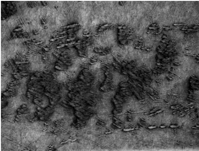
White-beam topograph of Si showing machining damages and strains
