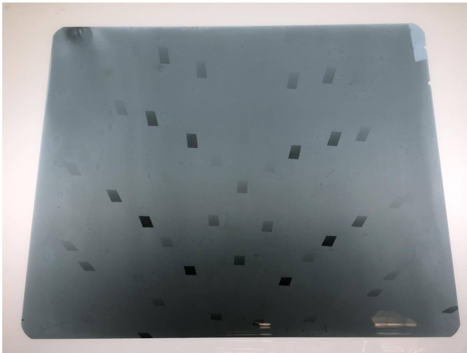
White-beam transmission Laue pattern recorded on X-ray film, each spot is a topograph
