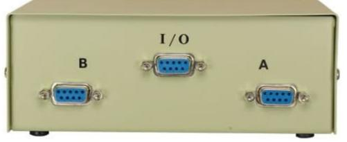
Rear view of switch box & connections
