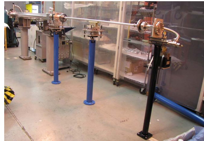
Fig. 3. HSCU and APS ID vacuum chambers are assembled at the APS vacuum shop
