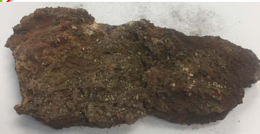
Large flakes that have fallen off the OD of the LTHW carrier pipe, showing corroded carbon steel mixed with matted (wet) insulation (above and right)
