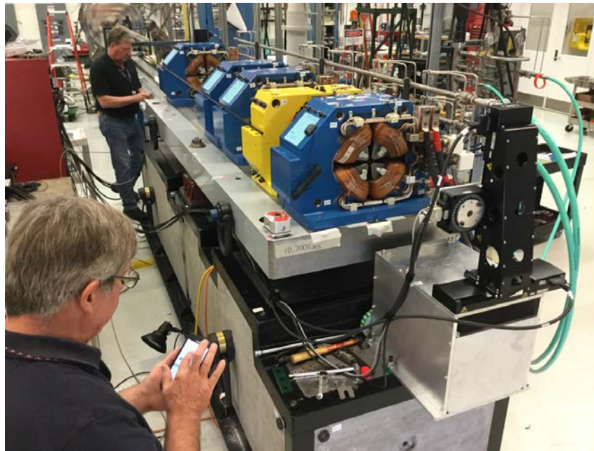
APS-U DMM magnets on the magnet measurement test stand
