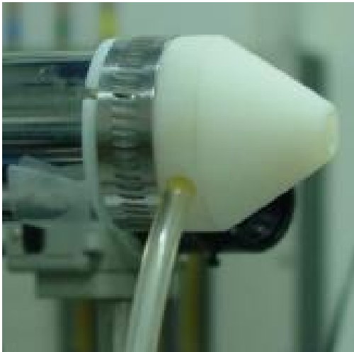
Collimator piece replacing wire EDM processing with 3D printing
