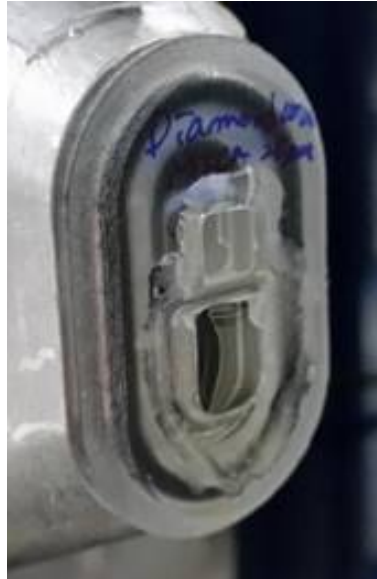
Window at the end of SAXS chamber (Sector 12), gasket printed integrally to part
