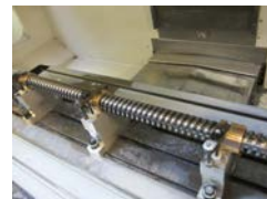
Machining of a helical SCU core
