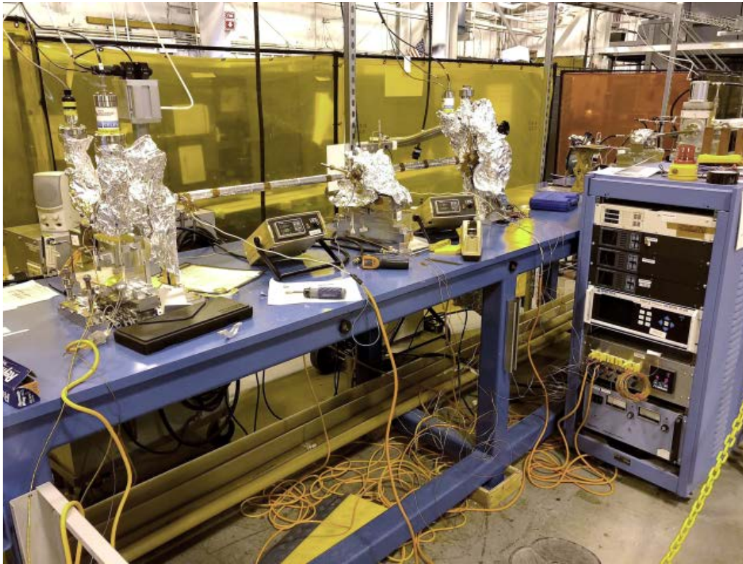
Vacuum Section undergoing bakeout testing
