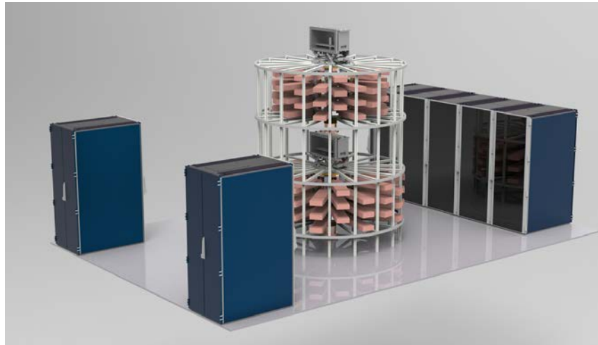
Conceptual layout of 200-kW SSPA rf station occupying the same floor space as klystron.
