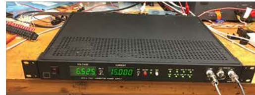
In-House Design Fast Bipolar Power Supply*
