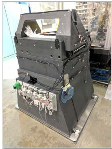
Velociprobe: fast scanning nano-probe
