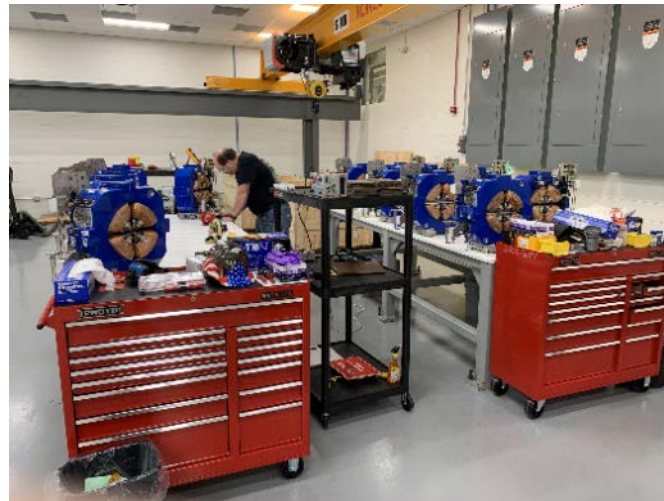
AES support of APS-U with the mechanical inspection, hi-pot, hydrostatic testing, and flowrate measurements on magnets
