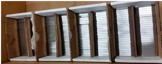
First batch of poles for the 2.8cm period undulator after machining and prior to heat treatment
