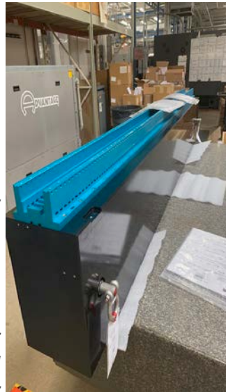
First batch of poles for the 2.8cm period undulator after machining and prior to heat treatment
