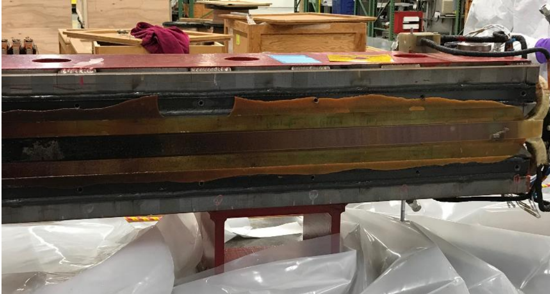
Discoloration noted in magnet coil/epoxy assembly after side plate removed on first failed injection septum magnet
