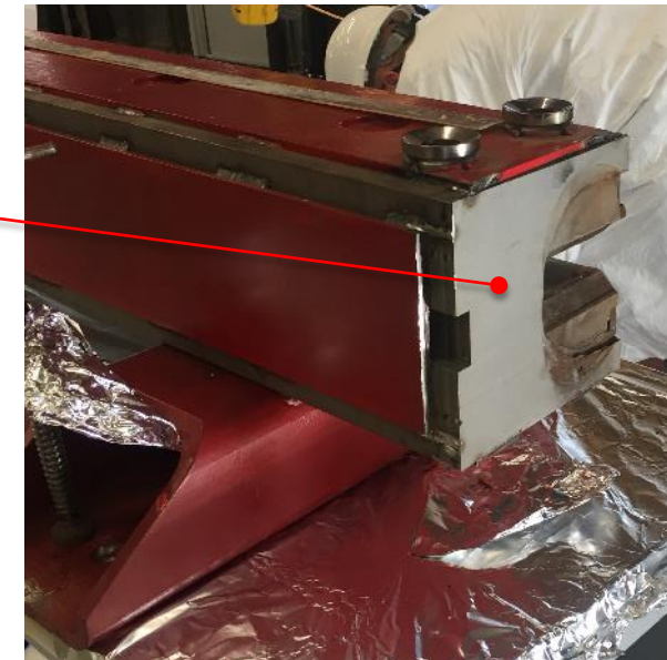
Machined end of septum, showing location of separated, broken laminations
