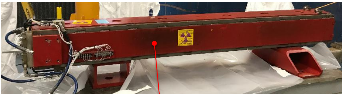
Discoloration noted on plate opposite of removed side plate, on first failed injection septum magnet
