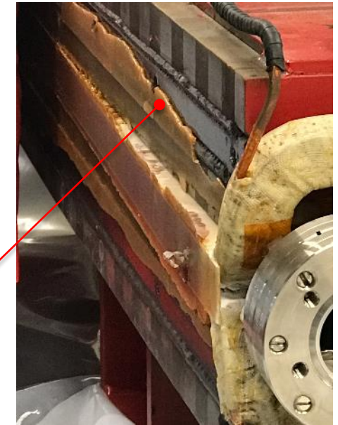
Mechanical separation of epoxy from magnet core
