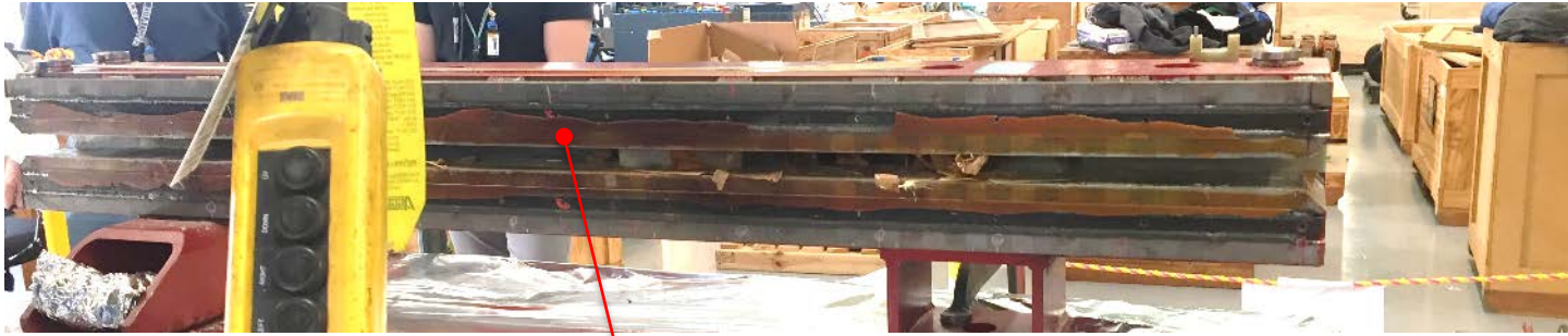
Discoloration with magnet coil, epoxy, chamber removed from core
