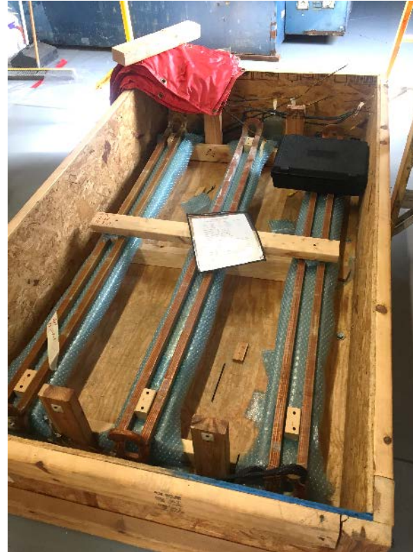
Spare septum magnet coils (3) in spare stock, from circa March 2004
