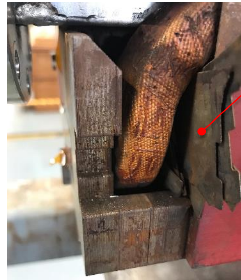
Loose laminations as-found on first failed septum
