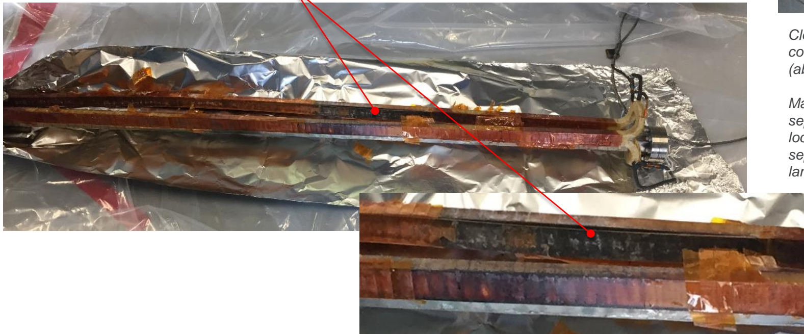
Separation of laminations and discoloration corresponding to location in image above
