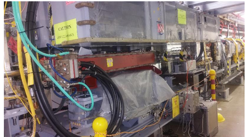
Upstream and downstream views of S:IS1 injection septum magnet Photos courtesy Cassandra Hayden
