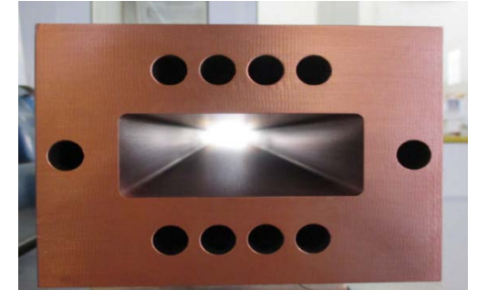
Glidcop bodies for the high heat load front end masks after polishing of the inner surface.
