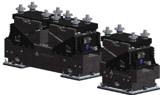
Picture of parts for the bases of the ASL mirrors at vendor, and solid model of what the assembled bases will look like.
