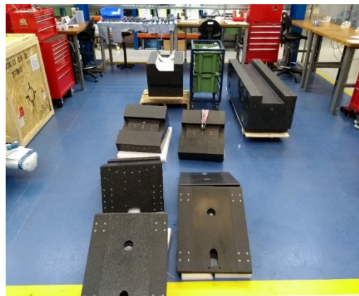
Picture of parts for the bases of the ASL mirrors at vendor, and solid model of what the assembled bases will look like.
