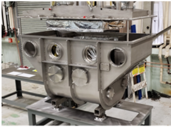
SC bunch lengthening cavity and cryo-vessel
