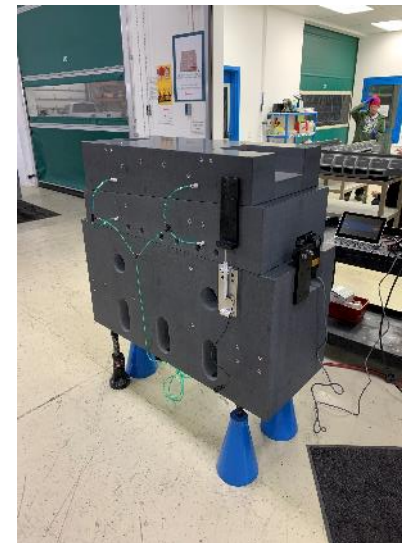
CU front end tables (left), CU front end spool pieces undergoing FAT (middle two) and the granite base for the CU GRID XBPM support system undergoing FAT (right).
