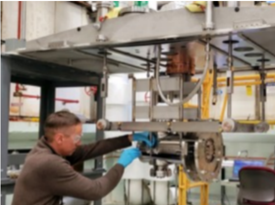
SC bunch lengthening cavity and cryo-vessel
