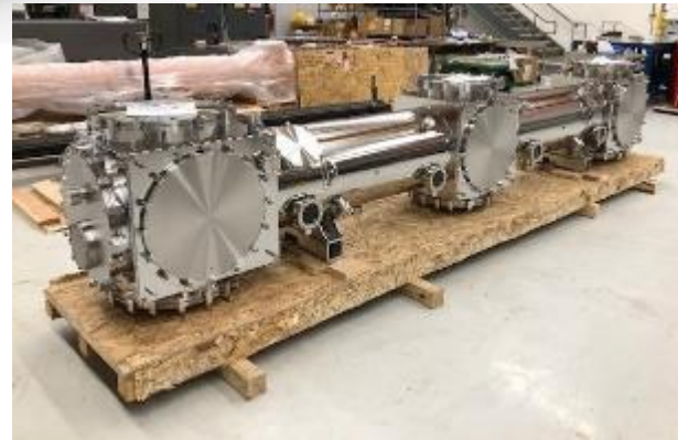
SCU Cryostat delivered to ANL
