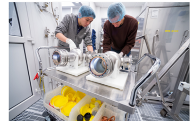
Superconducting bunch lengthening cavities
