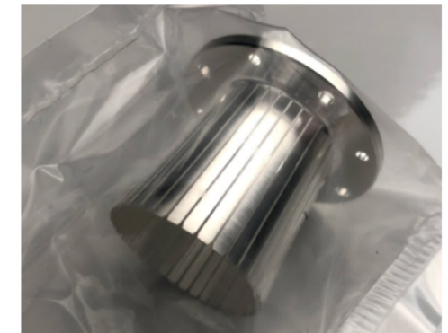
Figure 10: A silver-plated Glidcop rf liner.
