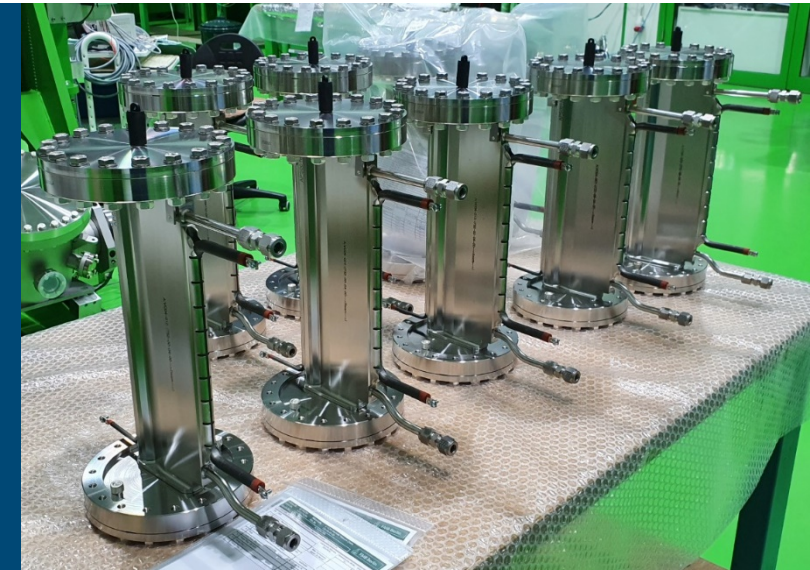
A set of the first production batch (40 total) of keyhole vacuum chambers prior to shipment from the vendor.
