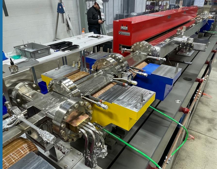
*Vacuum chamber insertion in a DLM-A module*
