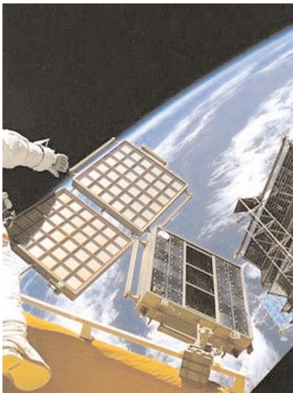
FIG. 1. Particle collector tray exposed on the MIR Space Station (NASA photo).
