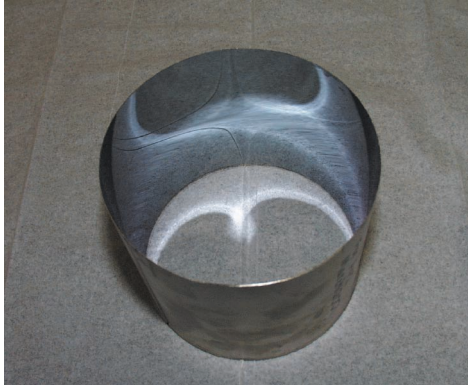
FIG. 1. W/Si multilayer coated mirror made by the IEMP process.
