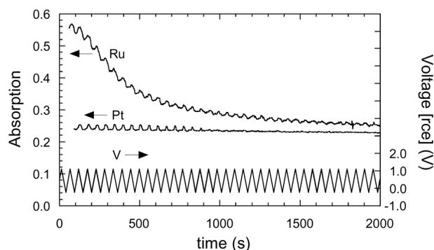
FIG. 1. Plots of Ru and Pt absorption versus time for voltage cycling between -0.25 and 1.10 V (rce) at 50 mV/s for a 1 M CH<sub>3</sub>OH + 0.5 M H<sub>2</sub>SO<sub>4</sub> solution.
