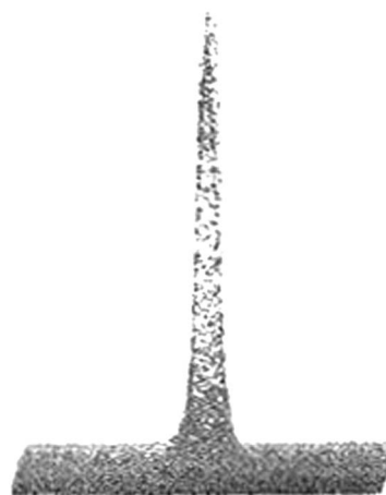
FIG. 4. 2-D image of the focal spot of the 9.1-keV focus at L_2 = 116 cm.
